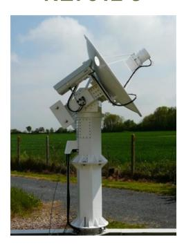
This station is designed for signals Receive in S frequency band.
