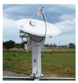
This station is designed for signals Receive in S frequency band.
