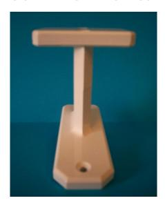
This antenna operating in L frequency band has been designed for working in horizontal
